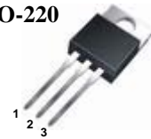
1.Gate 2. Drain 3. Source
