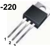
1.Gate 2. Drain 3. Source
