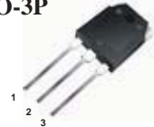
1.Gate 2. Drain 3. Source
